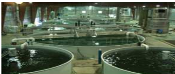
Closed tank re-circulation system in W. Virginia PHOTO: Blue Ridge Aquaculture
